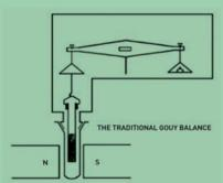
The traditional technique, developed by Gouy, employs a conventional balance and a large permanent magnet. The magnet remains stationary while the sample is caused to move, giving apparent gain or loss in sample weight
